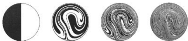
Figure 1. Typical mixture plots obtained for a global chaotic flow stirring protocol at the exit of bends 8, 16 and 24, at a low Reynolds number in a twisted pipes mixer (numerical experiments by Le Guer and Schall, 2004).
